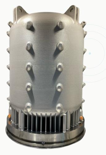
Orbiter propellant tank: Titanium pressure vessel printed in Ti-6Al4V shown as printed still attached to the build plate. Printed as a single piece, engineers can quickly have a fully functional assembly that is lighter, stronger, and reduces the risk for leaks.
