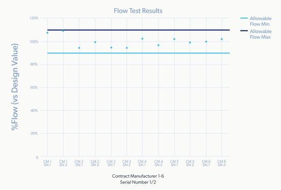
Flow test results demonstrating the consistent part performance for the test choke valve trims. The upper/lower flow criteria implies a dimensional accuracy of the internal channels which are  $\pm 0.002$ " (50 microns). These results underscore the quality and repeatability achievable with the Velo3D solution when working with CMs who are knowledgeable about the metal AM process.
