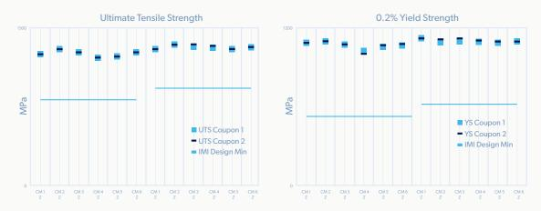
The plot shows how the static mechanical properties for the builds maintained an acceptable spread and met IMI specifications. For reference, each build was tested twice in XY and twice in Z directions for UTS and Yield strength, per APO20S AMSL Level 3.
