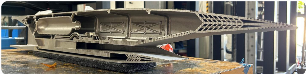
Printed cross-section of the AMUSER vehicle on a Velo3D Sapphire XC 1MZ
